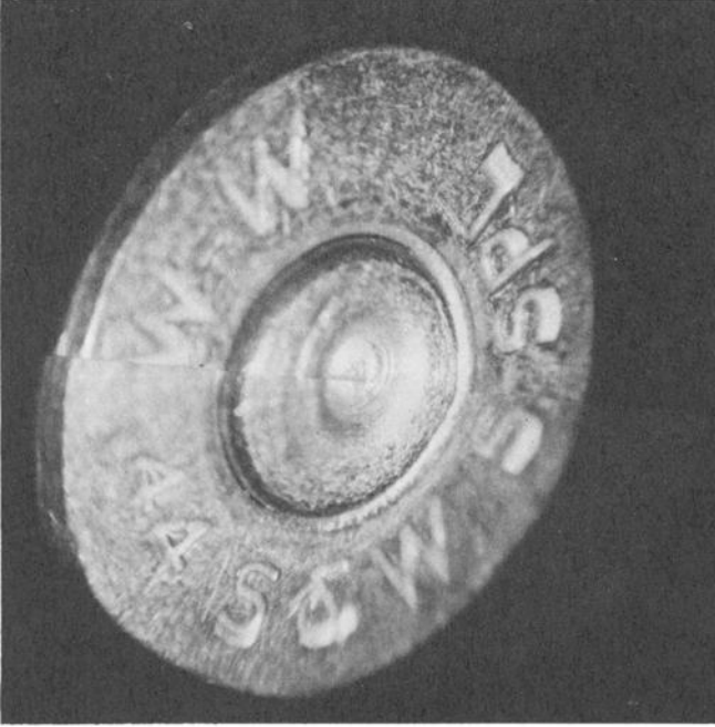
FIG. 10—Photomicrograph of two caliber .44 Special cartridge cases following discharge from Pen Gun F showing comparison of firing pin impressions and breech face marks suitable for positive identification (original magnification \times 4 , AFIP Neg. 74-6606-8).
